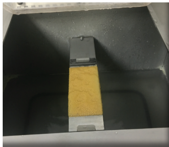
Figure 5: Water spray test
