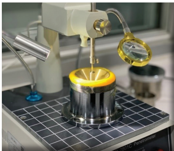
Figure 4: Penetration test (ASTM D217)
