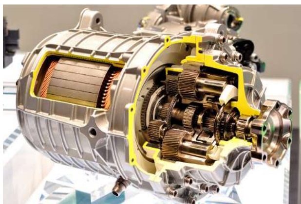
Integration of e-motor in transmission
